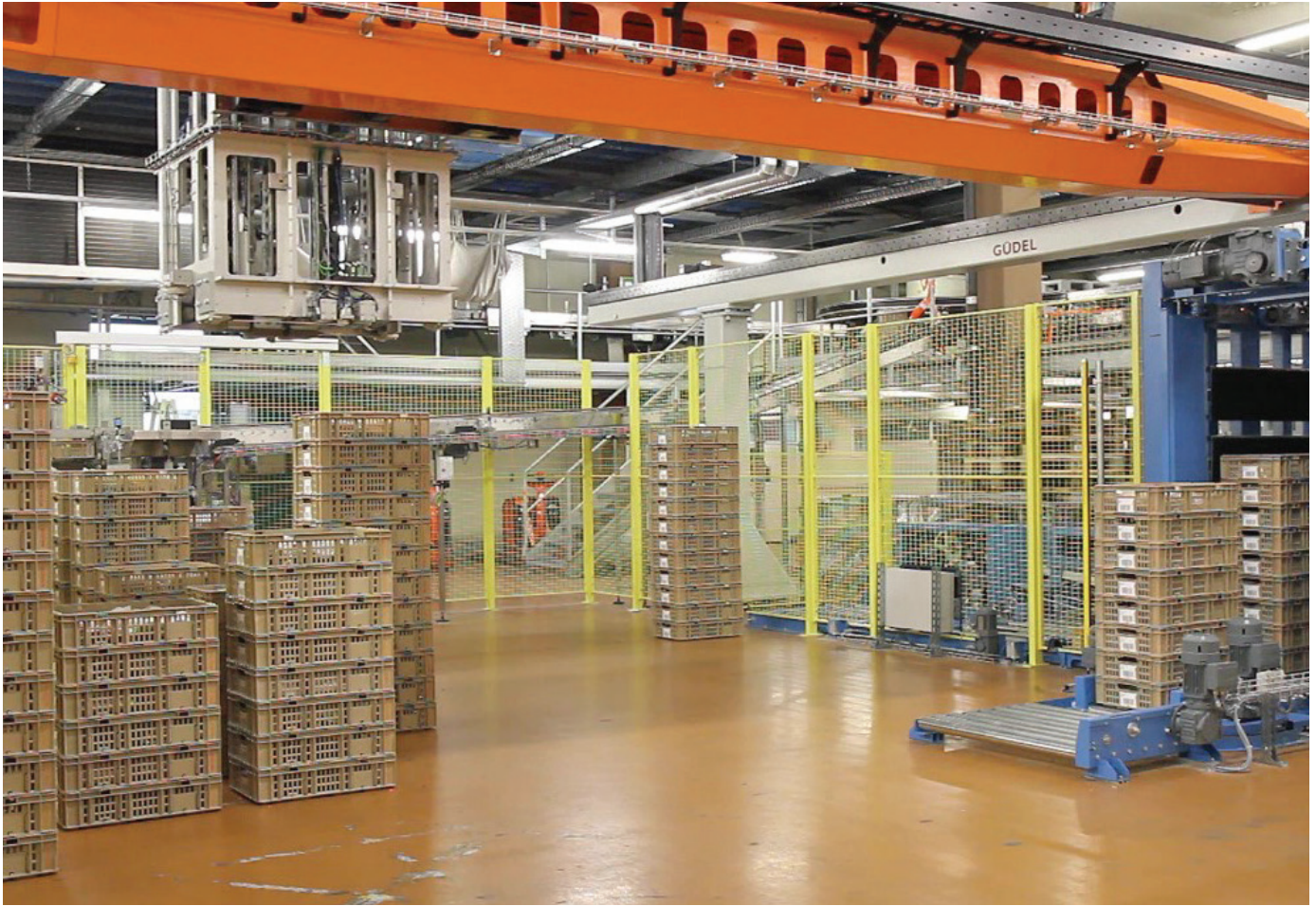
Güdel track modules and gantry products are commonly found in packaged food automation systems, such as palletizing work cells to extend the reach of the robot.
