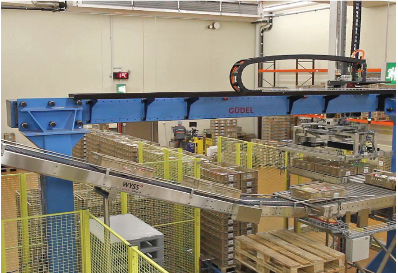
Güdel gantry solutions provide area coverage through overhead material handling large payloads.
